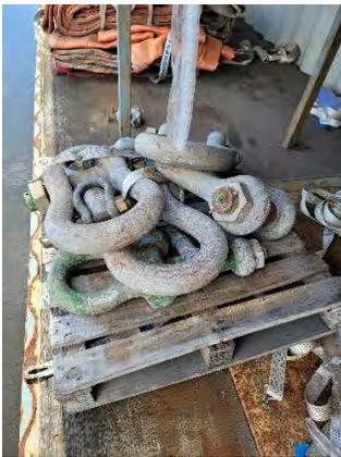
Shackles – U-Shaped Fastening device to link lifting gear together (grommets, slings, etc.)
