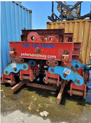
Equalizing Plates – Used for large yacht lifts to stabilize the lifting slings to keep them all the same length for lift.
