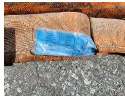
All round slings must have properly attached, legible tags with load capacities.
