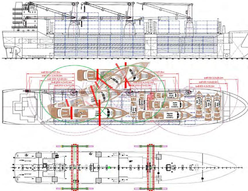
Stow plans and lifting plans prepared well in advance of loading / discharge.
