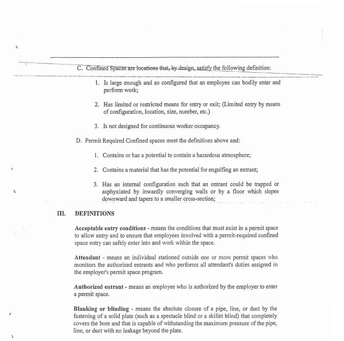
**Confined space** - means a space that (1) Is large enough and so configured that an employee can bodily enter and perform assigned work; and (2) Has limited or restricted means for entry or exit (for example, tanks, vessels, silos, storage bins, hoppers, vaults, and pits are spaces that may have limited means of entry.); and (3) Is not designed for continuous employee occupancy.
