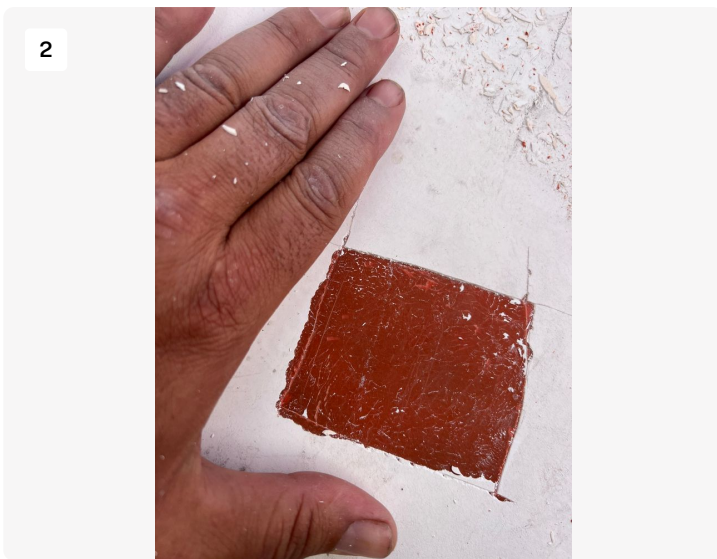
Spot in red slide, scraped off with a 5-1 multi tool. Minimal sanding marks.
