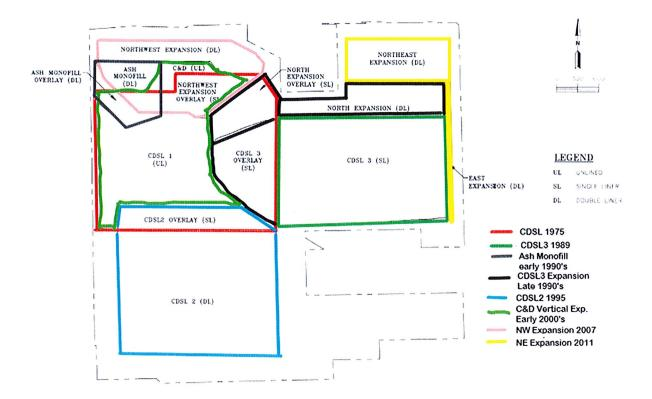
The area outlined in red, labeled "CDSL 1975 (UL)", is the original waste disposal area at the Central Disposal Sanitary Landfill (now known as the Monarch Hill Landfill). As indicated by the "UL" designation, this area is unlined; there is no liner to prevent contaminations from leaking directly from the garbage into the soil and groundwater. In many instances, waste was placed directly into the groundwater in this unlined area.
