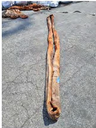
Endless Round Slings – load bearing, polyester woven yarn in tubular protective jacket used for lifting and connecting lifting equipment.
