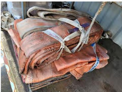
Boat Web Slings – Used to be place under the boat in proper cradle position, to lift boat or gear.
