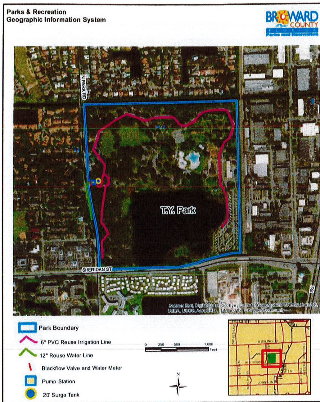
Figure 1. Proposed reclaimed water irrigation system for T.Y. Park.
