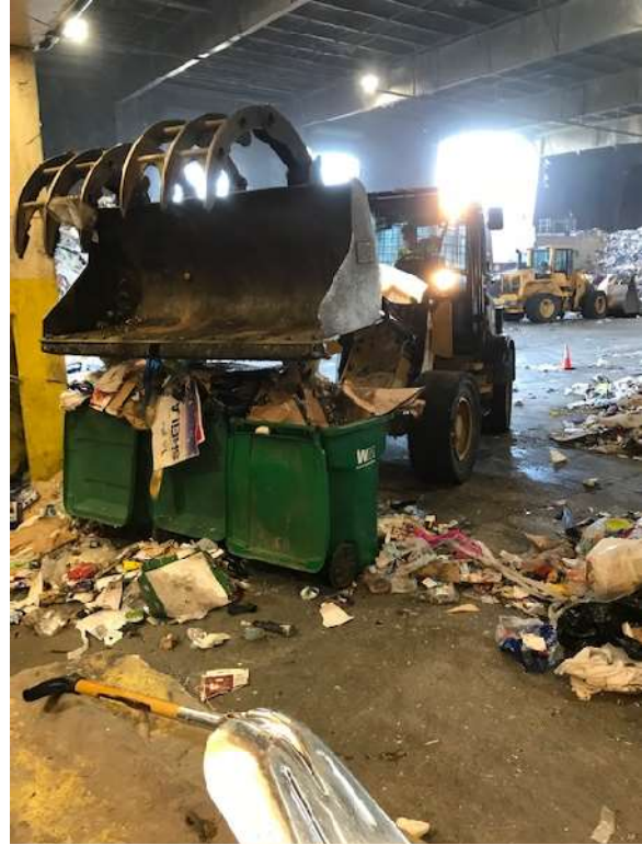
Loader Conveying Recycling Samples Into Holding Container
