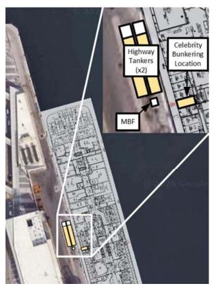
These graphics shows the ship alignment of its methanol bunker station with the anticipated layout of the MBF with two HTs connected. It also illustrates the access points on the ship used in SIMOPS. The distance from the northern point of the passenger bridges to the bunker site is approximately 105 ft. The approximately length of the HT and tractor is about 60 ft.
