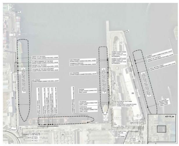
Figure 5-3. CT18, CT19, CT21, and CT25 Enlarged Electrical Site Plan (Sheet E112)
